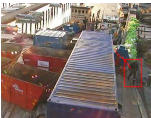
Intruder Detection: Vi-System rule "Person moving in an area" detects movement by unauthorized person in restricted area
